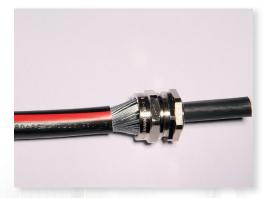
7. "Flare-up" the armouring and slide the gland over the flared armouring, making sure that the cone makes good contact with the armouring.
