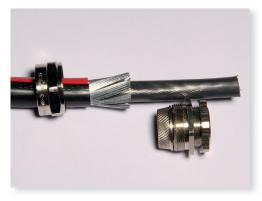
6. Measure approximately the distance of the cable required for the gland entry. Slide the gland nut over the cable, and cut the section of the sheathing that is required to enter the gland.
