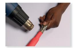
5. If you're covering a long length of cable with tubing, begin shrinking at one end, and gradually work your way down to the other. To ensure that the tubing shrinks evenly and without air bubbles, rotate the object as you're applying heat.
