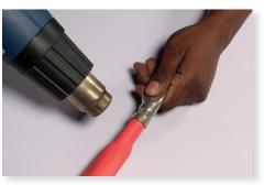
6. Evenly apply heat over the length and around the diameter of the tubing, until it is uniformly shrunken and conforms to the shape of the cable, hose, or splice that it's covering. Immediately remove the heat source, and allow the tubing to cool slowly before you apply physical stress to it.
