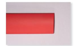
2. Cut the heat shrink tubing to a usable length (when cutting make sure you have clean and straight ends to avoid the tubing from splitting at the ends), and be sure to allow for a minimum 5-6mm overlap over any existing insulation or connectors. Keep in mind that tubing also shrinks lengthwise... typically 5-7% during the shrinking process.
