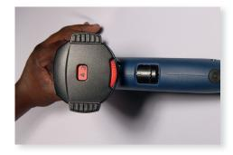
4. Before shrinking, check your tubing's specifications for the recommended heating temperature. Use a recommended heat gun to shrink the tubing. Since uncontrolled heat can cause uneven shrinkage, physical damage and insulation failure, the use of open flame is not recommended.
