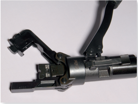
9. Insert the die in the die-head of the crimping tool.
