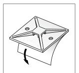
2. Peel off protective backing and ensure the adhesive area is not touched.
