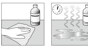
The surface must be dry, free from dust, oil, oxides, parting agents and other impurities. The surface to be glued should be cleaned using a clean cloth and isopropanol/water (50/50). When using other appropriate cleaning agents, ensure that they do not attack the surface nor leave any residues. After cleaning allow the surface to air-dry completely.
